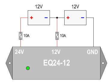
▲ CAUTION: Always disconnect or turn OFF all external charging sources and/or DC loads before installing or removing the EQ24-12 module.
